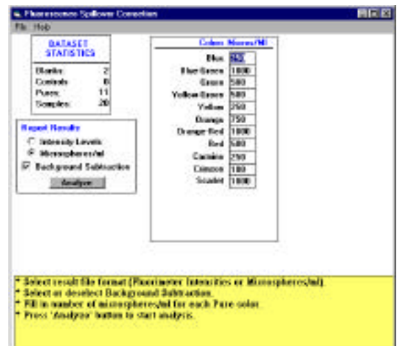
Figure 7: Screen display when results are requested in microspheres/ml. The microspheres/ml edit boxes must be filled out prior to continuing the
