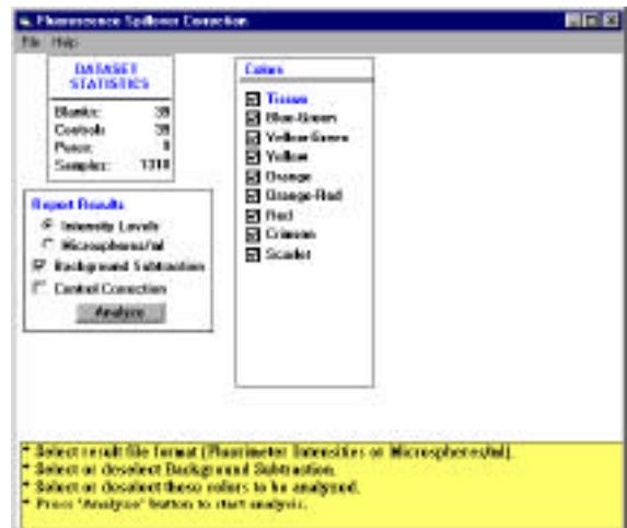
Figure 1: Initial screen for a fixed wavelength analysis. Defaults: (1) results are reported as intensity levels, (2) all wavelengths present are selected, (3) Background Subtraction is selected, and (4) Control Correction is disabled. Background Subtraction and Control Correction are present only if the appropriate files were selected during dataset selection.
